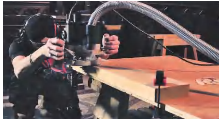
▲ Pic.7 Using the Trend T10 router to cut slots for the biscuits
